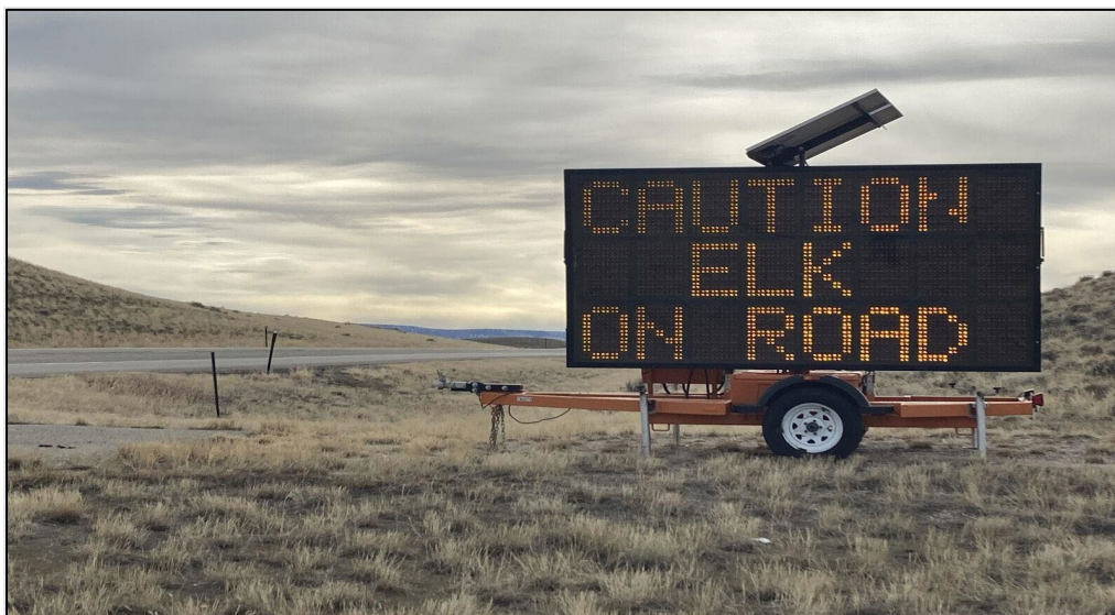
Typical message sign connected to an animal detection system to warn drivers of elk along the road. (komonews)
