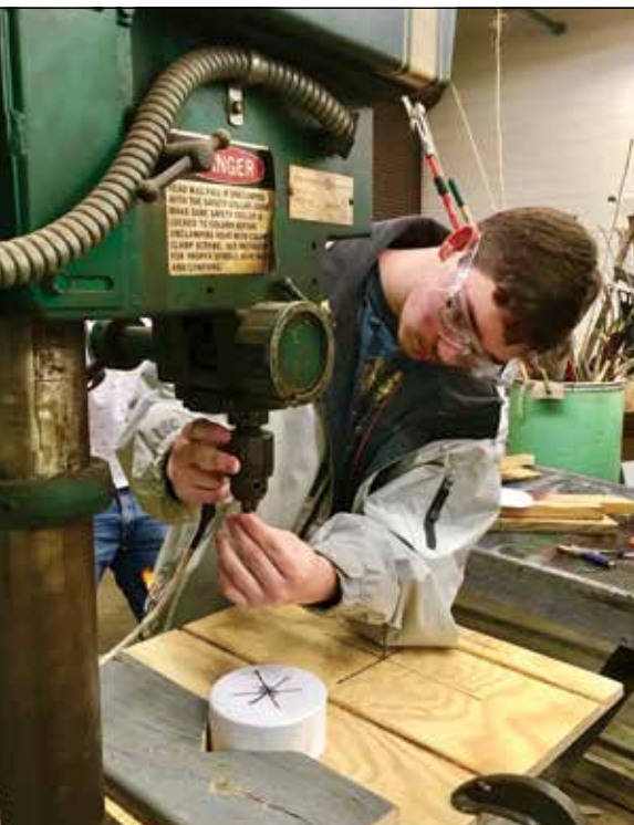
A Halifax County High School student sets up a press prior to drilling drain holes in a PVC nest bottom cap. Under teacher supervision, HCHS shop classes manufactured 50 of the project's nesting boxes.
